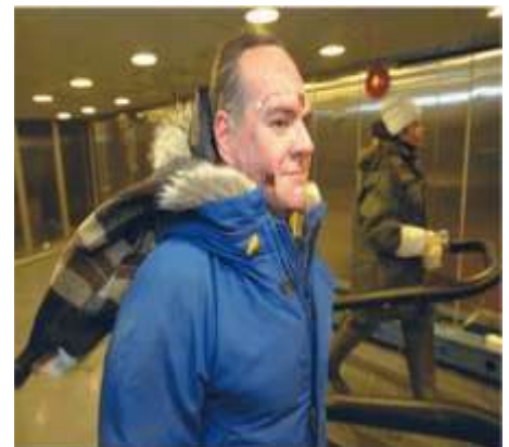
Wind chill test subjects walking on a treadmill in a chilled wind tunnel. Facial temperature readings were taken to help refine the new wind chill index.
